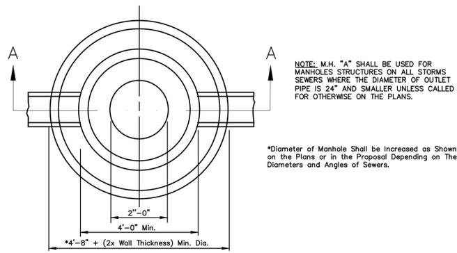
\*Diameter of Manhole Shall be Increased as Shown on the Plans or in the Proposal Depending on the Diameters and Angles of Sewers.
